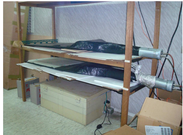
Fig. 2. Assembly of PMT, light guide, and scintillators.
