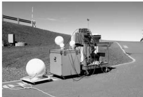
Fig. 1: The Bonner multisphere neutron spectrometer set in front of the Subaru Telescope on the top of the Mt. Mauna Kea.
