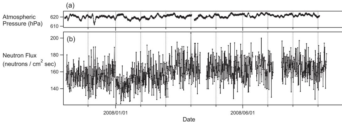
Fig. 2: Time dependence of the neutron flux measured in the building of Subaru Telescope. The flux is integrated from 8 to 1000 MeV. In trace (a), atmospheric pressure is also plotted.
