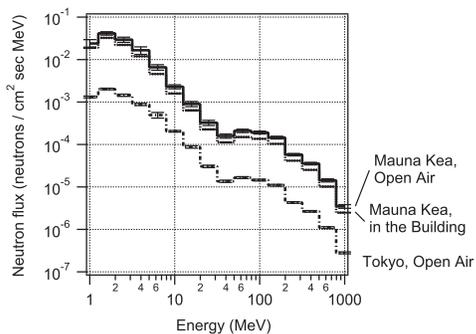
Fig. 3: Neutron energy spectra measured by Bonner multisphere spectrometer measured at the open air area and in the building of Subaru Telescope, and open air area of Tokyo.
