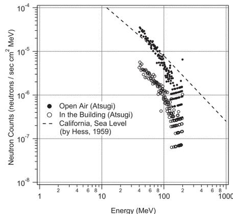
Fig. 4: Neutron energy spectra preliminary measured by scintillator spectrometer at Atsugi (Japan). Solid circles and open circles are measured at open air area and in the building, respectively. Dotted line indicates the spectrum reported by Hess *et al.* (1959) [1]
