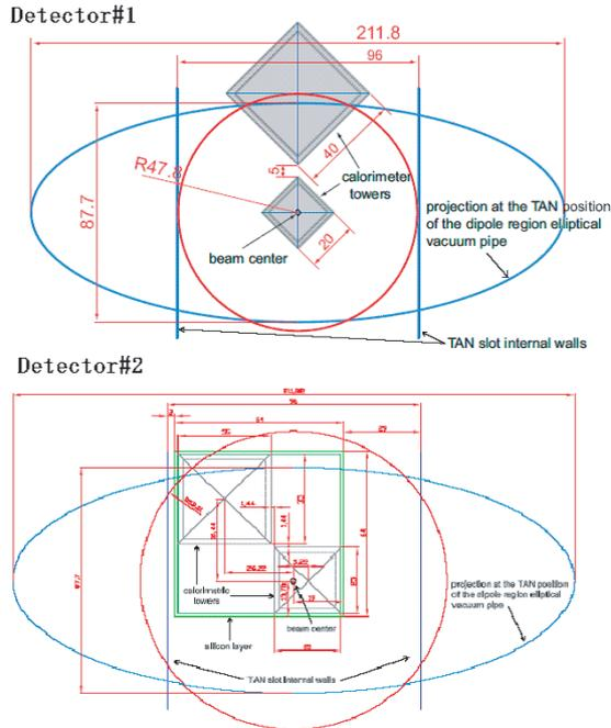
Fig. 5: The cross sections of the calorimeters. Top is the Arm1 calorimeter. Bottom is the Arm2 calorimeter.
