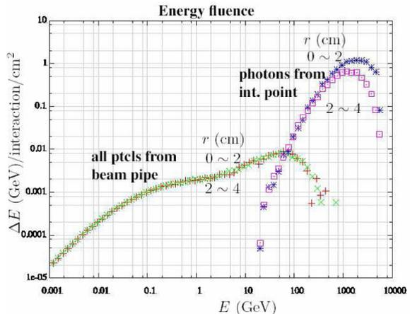
Fig. 2: The energy fluence of the beam pipe background and photons from IP at the calorimeter. Photons from IP dominate above 100 GeV while the background distribute below 100 GeV.
