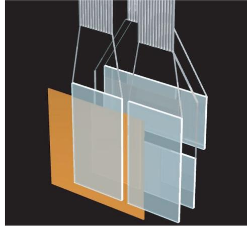
Fig. 6: A schematic view of The Front Counter. Two pairs of plastic scintillators segmented in vertical and horizontal directions. The size of a scintillator is  $4 \times 8$  cm. A  $8 \times 8$  cm copper plate of 0.5mm thickness is inserted between the pairs. The scintillator light outputs are fed to PMTs via an acrylic light guide and optical fibers.
