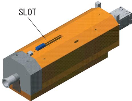
Fig. 1: The appearance of TAN absorber located 140 m from IP. It has an instrumentation slot 96 mm width.
