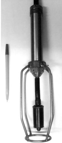
Fig. 2: Acoustic sensor with housed pre-amplifier and hydrophone H2020C.
