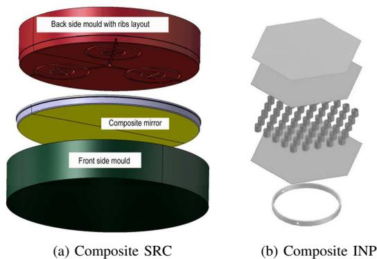
Fig. 2. (a) Composite mirror. The front and rear side steel moulds are pressed against the composite which retains the shape. The surface (yellow part) need aluminization and coating (b) Composite mirror from INP. From top to bottom: a spherical layer to be coated (cast on the front panel), the flat front panel, perforated tubes of uniform length interspacing front and rear panels, the flat rear panel and an example of mounting interface
