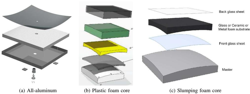
Fig. 1. (a) All-aluminum mirror. Two thin aluminum layers are sandwiched together with aeronautic glue, interspaced by a honeycomb layer. The surface is diamond-machined and quartz-protected. (b) Plastic-foam core mirror. From top to bottom: a glass-fiber envelope (or a glass-sheet), a pre-formed foam block, resin, a second glass-sheet and the spherical mould. (c) Cold-slumping foam-glass mirror.
