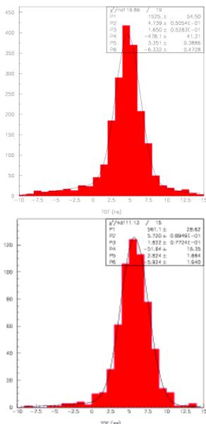
Fig. 6. The distribution of time of flight between the two  $20 \times 20 \text{ cm}^2$  tiles  $160 \text{ cm}$  apart, for downward vertical cosmic ray events (top) and diagonal (bottom). The towers are apart  $60 \text{ cm}$ .
