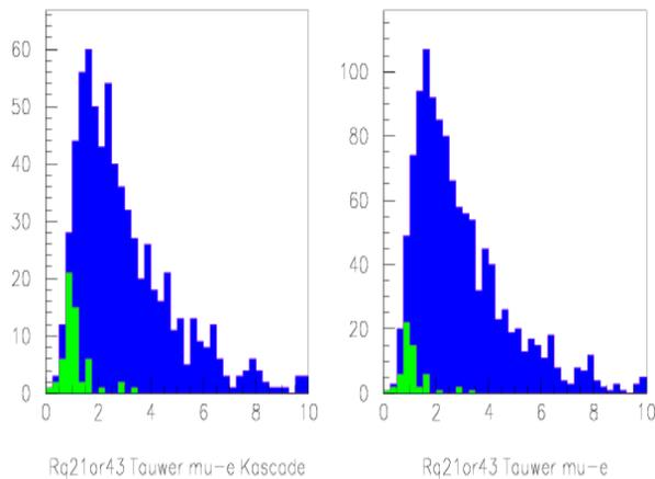
Fig. 8. Ratio of deposited energy on bottom tile to top tile for tracks having a TOF between  $2-8 \text{ ns}$ . Right: Electron (black) and muon (gray) are separated by criteria shown in sec. 2.0. Left: The same sample with KASCADE-Grande validation.
