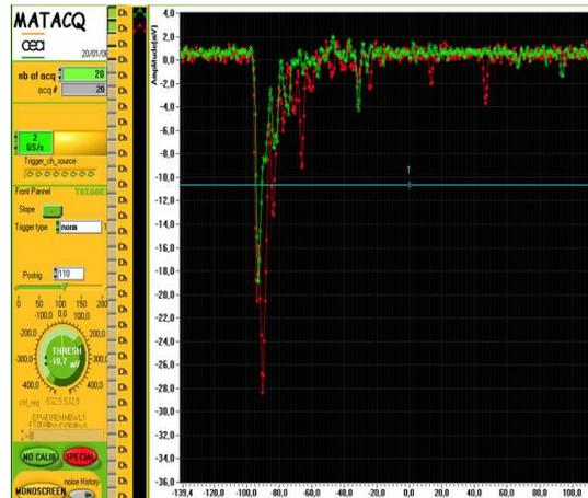
Fig. 2. Two photomultiplier signals of same tower displayed by Maticq board. The units are  $mV$  (vertical axis) and  $ns$  (horizontal axis). A square is  $2mV$  times  $20 ns$
