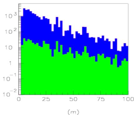
Fig. 7. Electron (black) and muon (gray) density per  $\text{m}^2$  versus distance from the core for reconstructed tracks by TOF in the interval  $2-8 \text{ ns}$ .
