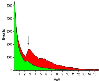
Fig. 5. Energy deposited by 200 MeV electron on the bottom tile covered by a layer of lead of 5 cm (gray) and 2.5 cm (black). The arrow shows the average of energy deposited on top tile.
