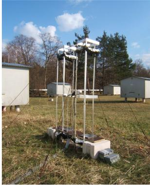
Fig. 3. Setup of the module. The layers of lead are on the bottom tile. The DAQ is located in the cluster room n.12.
