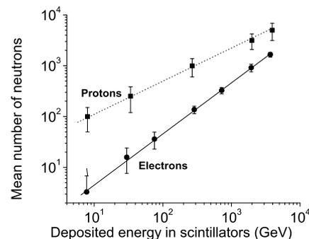
Fig. 3:  $N_{meas}$  in dependence on deposited energy in scintillators for incident protons and electrons, error bars denote standard deviations in every point.
