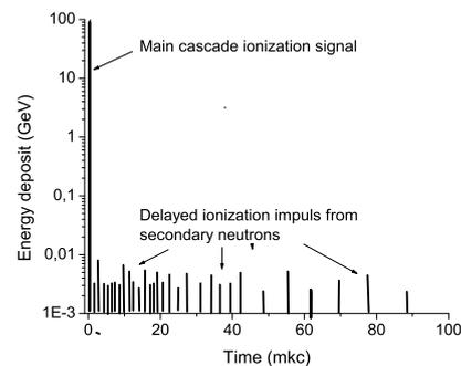
Fig. 1: Schematic view of the signal from incident particle with delayed ionization from secondary neutrons
