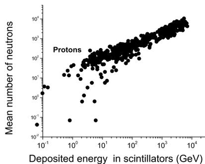
Fig. 4:  $N_{meas}$  versus deposited energy in scintillators for individual cascades at 50 GeV - 30 TeV
