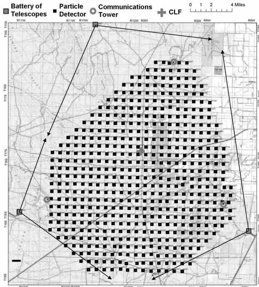
Fig. 1. Configuration of the TA detector, showing the positions of 507 deployed surface detectors surrounded by the three FD stations. The cross mark in the center of the TA site shows the position of the Central Laser Facility (CLF).
