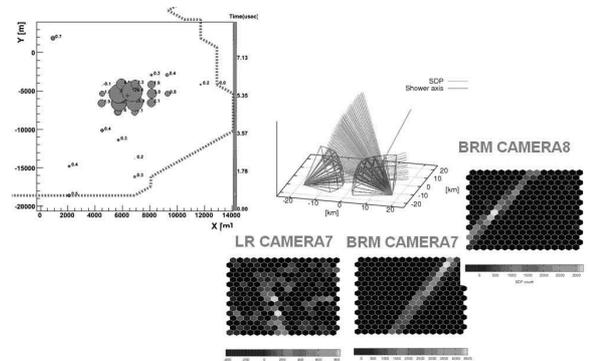
Fig. 3. An example of a hybrid stereo event. Left figure shows the data taken by the surface detectors. Right figure shows the shower reconstruction from the data taken by BRM FD and LR FD.
