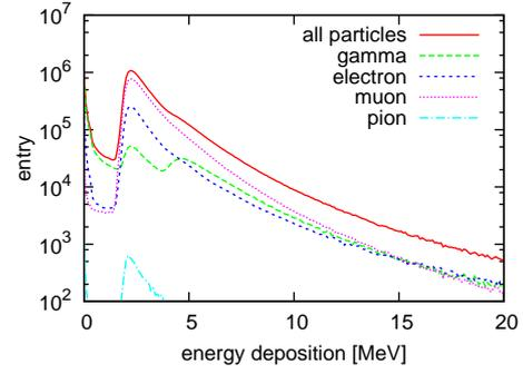
Fig. 2. Spectra of energy depositions by the simulation. solid-line : energy deposition spectrum by all particles, long-dashed-line : gamma rays, dashed-line : electrons, dotted-line : muons, chain-line : pions.
