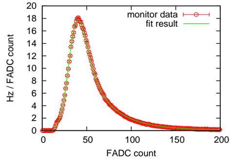
Fig. 3. Expected energy deposit by the simulation is shown by the solid line, and the measured spectrum is plotted by the open circle. The solid line is the result of fitting described in the text. The Detector gain of this counter was determined as 17.4 FADC counts per MeV energy deposit and the number of photo-electrons per MeV was estimated to be 20.4.
