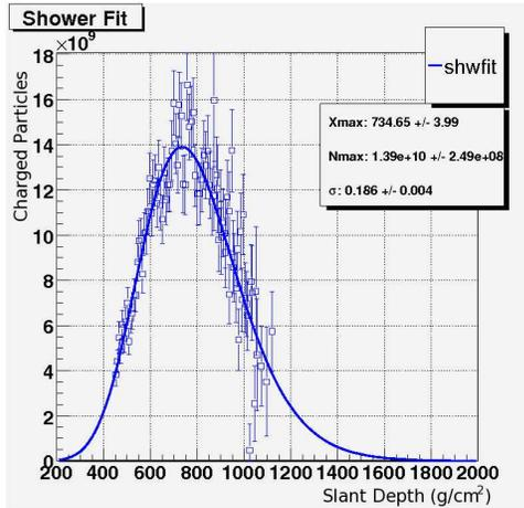
Fig. 2. Shower profile of HiRes stereoscopic event. Phototube pulses are sorted into time bins, the  $y$ -axis is converted from fluorescence light output (proportional to energy deposition) to the number of charged particles assuming an average energy deposition per particle of 2.4 MeV/g  $\text{cm}^2$ .
