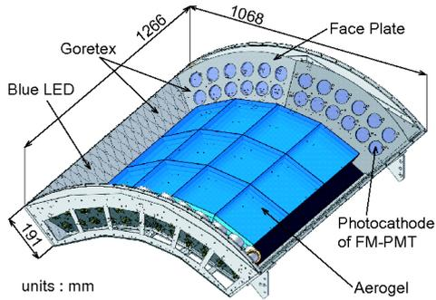
Fig. 4. Overview of the Aerogel Cherenkov counter.
