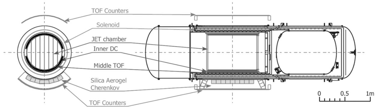
Fig. 2. Cross-sectional views of the BESS-Polar II payload
