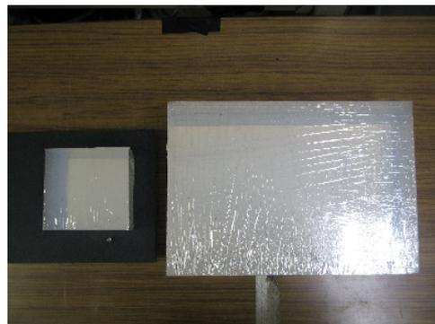
Fig. 3. Comparison aerogel block. Left block was used in Polar-I and right block was reproduced for Polar-II.
