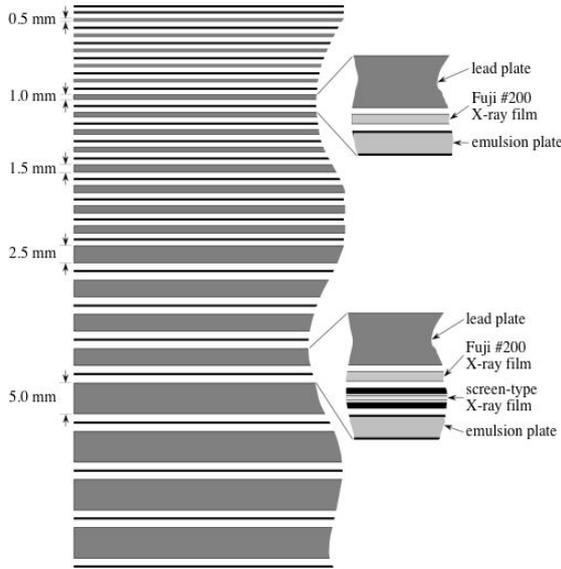
Fig. 1. The typical structure of emulsion chambers.
