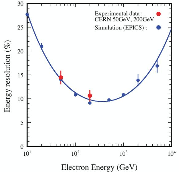
Fig. 3. Energy dependence of energy resolutions with the emulsion chambers for electrons of 50 GeV and 200 GeV, compared to the simulations.
