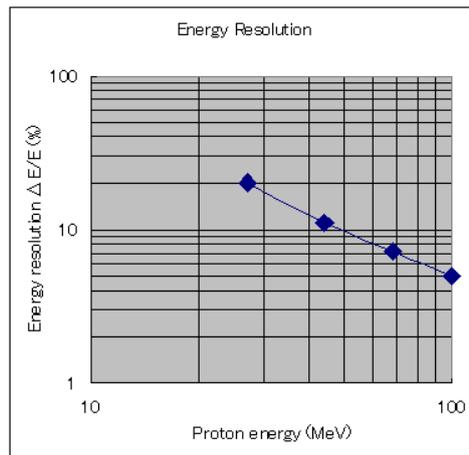
Fig. 2: The energy resolution of the neutron detector obtained using the range method is shown as a function of the energy of incoming protons. The energy resolution can be well fitted to a function of  $\Delta E/E=10\%/(E/50\text{MeV})$ .
