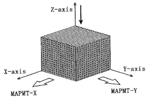
Fig. 1: Schematic view of the neutron detector. It comprises scintillation plates of  $3\text{mm} \times 6\text{mm} \times 96\text{mm}$ . The signal of each plate is read out by the multi-anode photomultipliers. The track pattern can be recognized using 512 data points. The total weight of the FIB detector is about 20kg, except the interface part.
