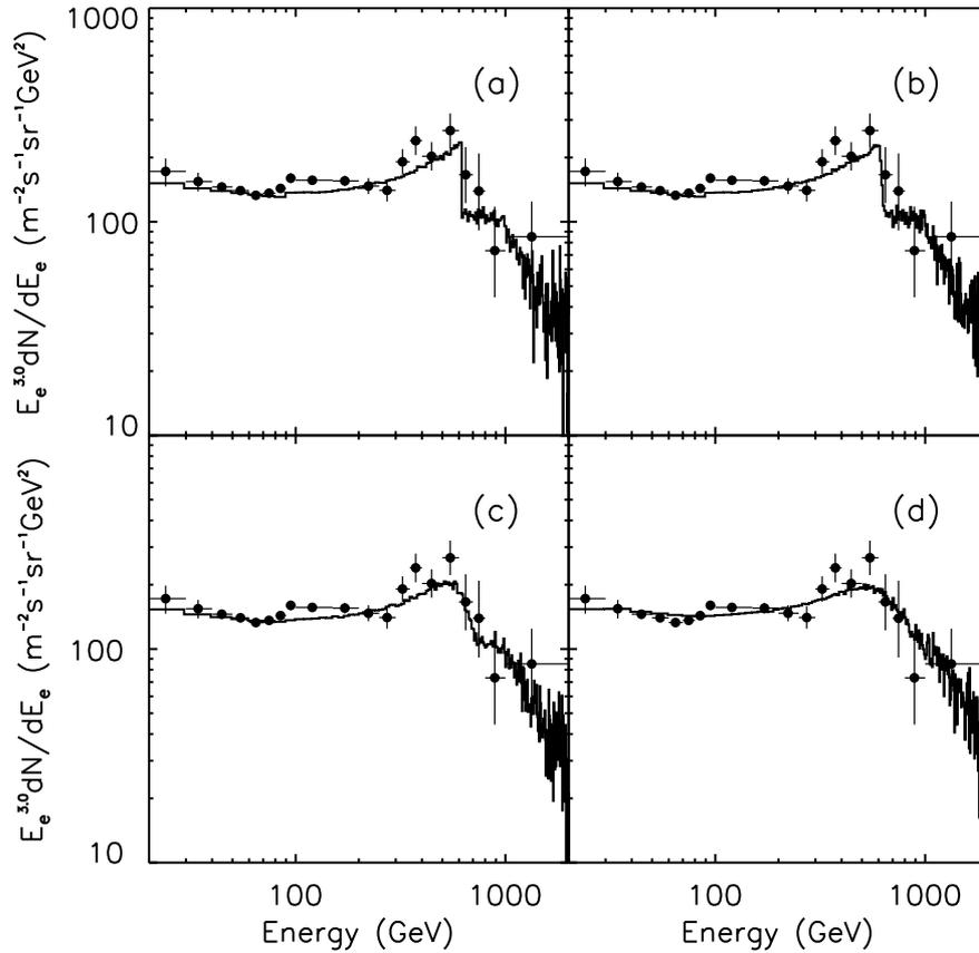
Fig. 1. The simulated high energy electron spectra observed by instruments with different energy resolution, a:input spectrum., b: energy resolution =1.5%,c: energy resolution =10%, d: energy resolution =25%.
