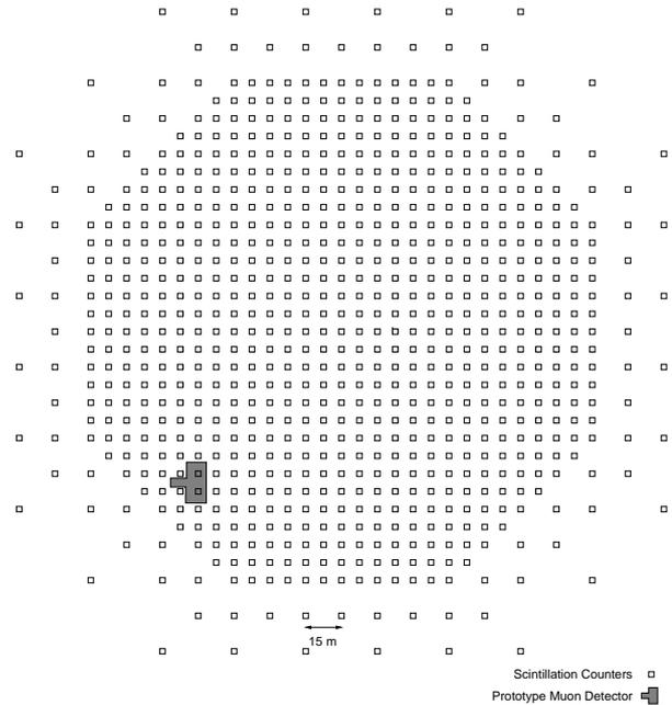
Fig. 1. The Tibet airshower array with scintillation counters (Open squares) and the 100 m<sup>2</sup> prototype water Cherenkov muon detector (Gray area).
