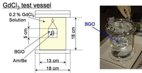
Fig. 4. The test vessel used for the neutron tagging efficiency measurements in SK.
