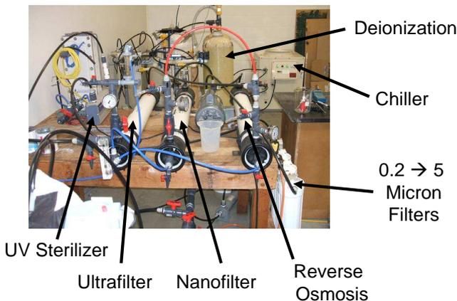
Fig. 3. The water purification system at UCI.
