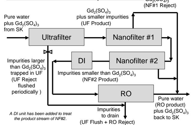
Fig. 2. The proposed water purification system.
