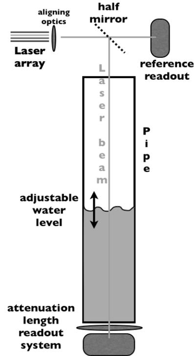
Fig. 1. The water transparency measurement device at UCI.
