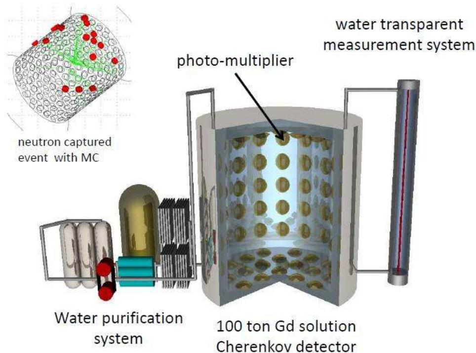
Fig. 6. A planned test facility for the Gd Cherenkov detector demonstration.
