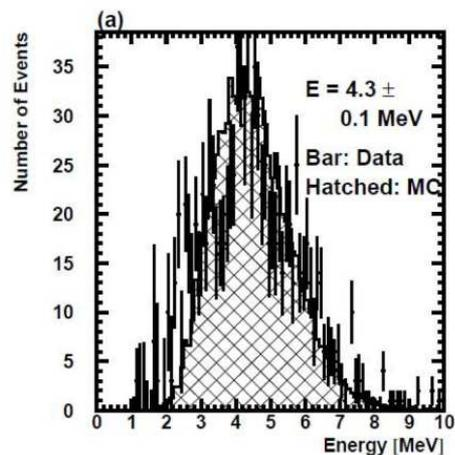
Fig. 5. The energy spectrum of the gamma rays from Gd capturing a neutron. The points with bars represent data, while the histogram shows the MC prediction.
