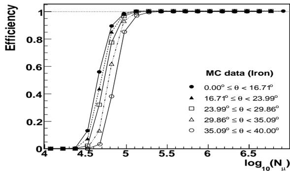
Fig. 1: KASCADE-Grande triggering and reconstruction efficiency shown as a function of the muon number for different zenith angle intervals. The efficiency was estimated from MC simulations assuming a pure iron composition.
