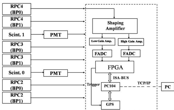
Fig. 2: Schematic diagram of the electronics and DAQ.
