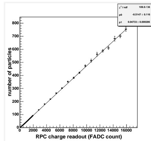
Fig. 6: Number of charged particles VS. RPC charge readout, a linear fit is performed to the data.
