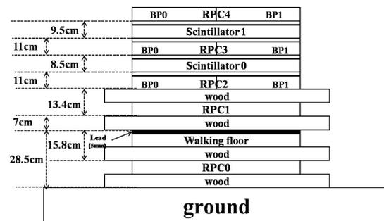
Fig. 1: Sketch map of the calibration telescope. Three RPCs (RPC2, RPC3, RPC4) act as the detectors to be calibrated.
