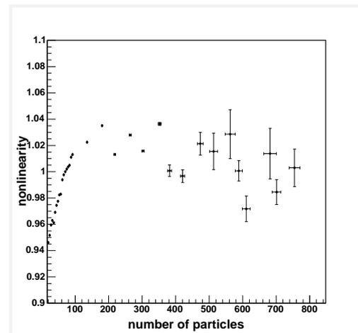
Fig. 7: Nonlinearity of the calibration.
