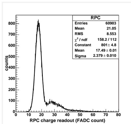
Fig. 5: Charge readout of one RPC in case of single particles. The black curve presents a Gaussian fit to the single streamer peak.
