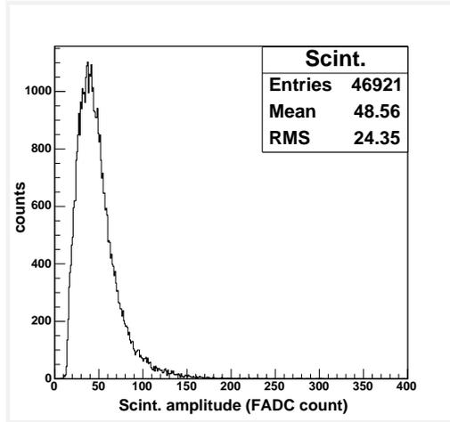
Fig. 4: Amplitude distribution of one scintillation detector in case of single particles (HV=610V).
