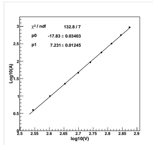
Fig. 3: High Voltage response of one PMT, superposed with a linear fit.
