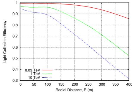
Fig. 2: Comparison of light detection for a finite  $FoV$  and an infinite  $FoV$  as a function of impact parameter. Y-axis shows the ratio of light collection efficiency of a finite  $FoV$  to the efficiency of the infinite  $FoV$ .
