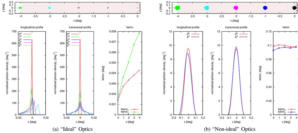
Fig. 3: Scatter plots for Cherenkov light in the detector plane (upper panels) and FWHM plots (bottom panels) are shown for different angular offsets of the light source.
