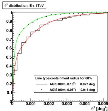
Fig. 5: Angular resolutions for  $0.1^\circ$  and  $0.05^\circ$  pixel sizes in the approximation of infinite array with spacing 100 m.
