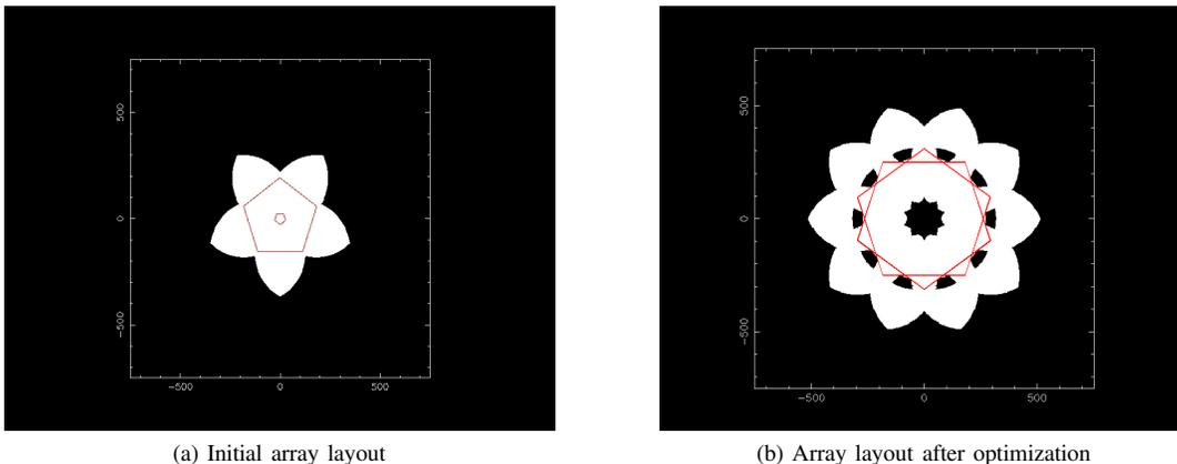
Fig. 1: Optimization of the array consisting of two concentric cells. The white areas indicate the regions where showers would deliver signals above the threshold to at least 2 telescopes and the angle between the lines connecting these telescopes and the shower core is greater than  $\sim 30^\circ$ .
