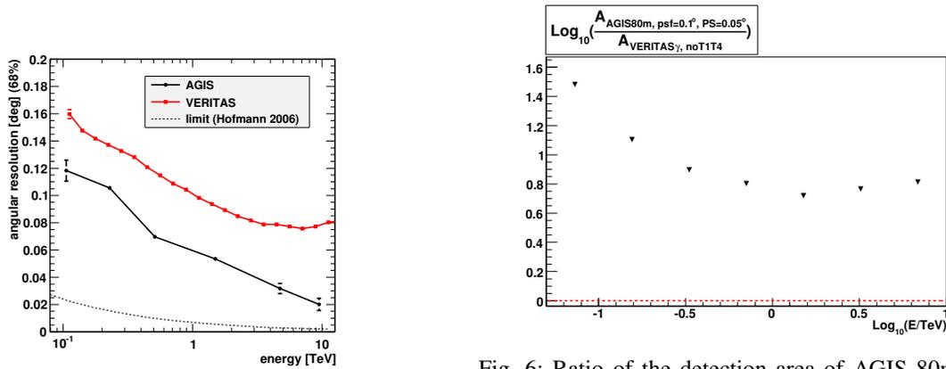
Fig. 4: Angular resolution (with  $0.1^\circ$  camera pixels) vs. energy for a 36 telescope array with telescope distances of 125m compared with VERITAS [8] and the theoretical limit as derived in [9].
