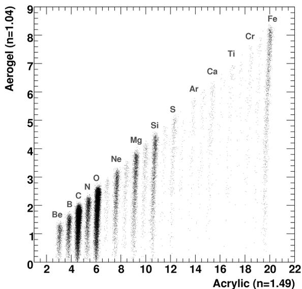
Fig. 4. Response of a combination of aerogel and acrylic Cherenkov counters to a simulated flux of cosmic-ray nuclei.
