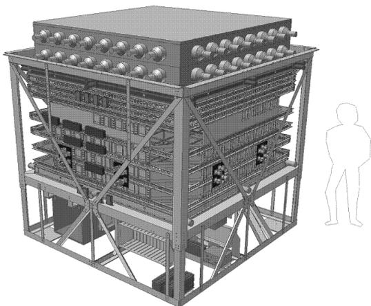
Fig. 2. Combination of TRACER with two Cherenkov counters in light-integration boxes.
