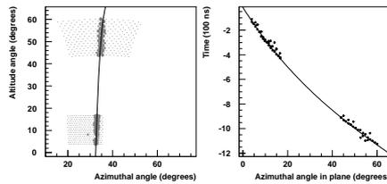
Fig. 2. Event seen in both the TALE Tower prototype and the HiRes-I detector. *Left panel:* Image of a cosmic-ray event in altitude and azimuth as seen by the Tower and a HiRes-I mirror. *Right panel:* Time vs. angle plot with best-fit event geometry overlaid. The impact parameter for this event was found to be  $3.82 \pm 0.04$  km.
