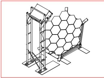
Fig. 1. Drawing of the TALE Tower detector prototype.
