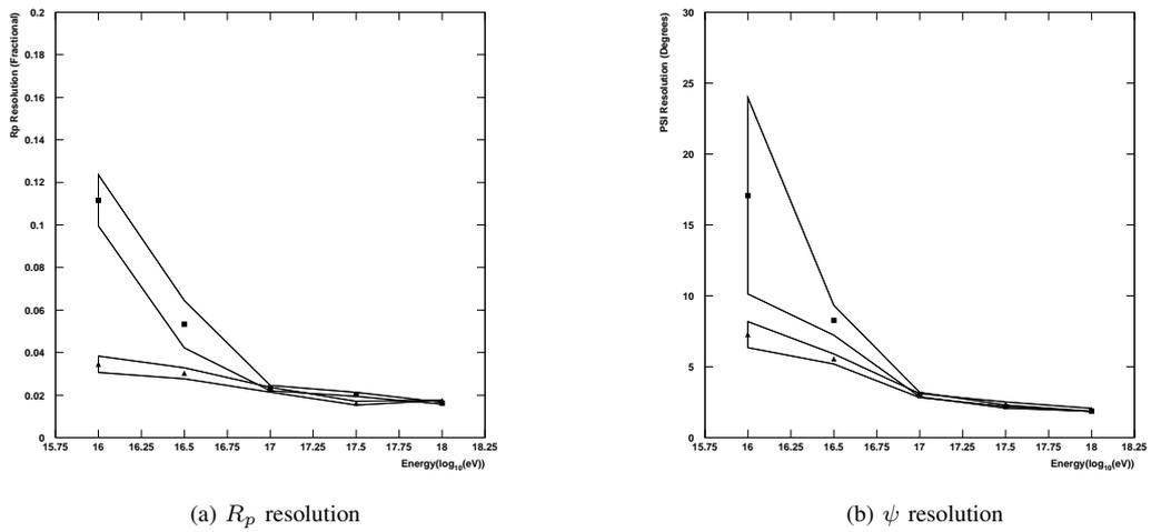
Fig. 3. Resolution for reconstructing the impact parameter,  $R_p$  and the angle in the shower-detector plane,  $\psi$  from simulations using an FADC with a 100-ns sampling rate (*squares*) and a 25-ns sampling rate (*triangles*). The ability to reconstruct cosmic rays with energies less than about  $10^{17}$  eV is greatly enhanced using a 25-ns sampling rate.
