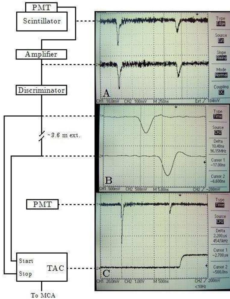
Fig. 1: Left: Schematic of selected experiment. Right: Actual measured voltage of **A**: PMT and amplified PMT pulse pair, **B**: TAC stop and start inputs, **C**: TAC output with PMT pulse pair. The oscilloscope readings are to illustrate PMT amplification, the delay in the start pulse sent to the TAC, and a typical calibration measurement.
