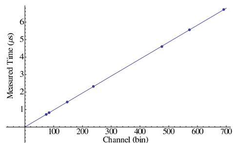
Fig. 2: Time to MCA channel calibration example. Each point represents a muon decay.
