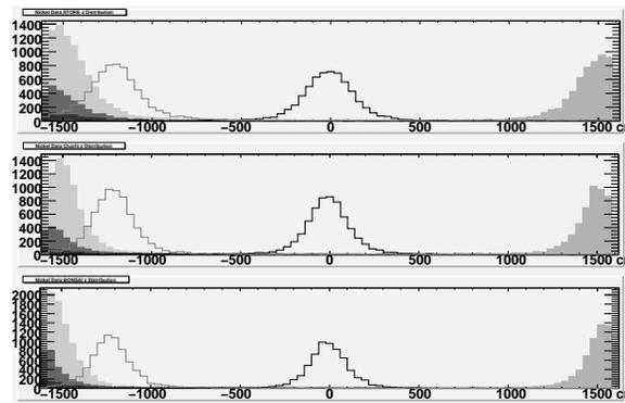
Fig. 4. Test of WIT System with Ni-Cf Calibration Source at Six Positions: (0.4,-0.7,-17.1)m,(0.4,-0.7,-16.1)m, (0.4,-0.7,-15.1)m, (0.4,-0.7,-12)m, (0.4,-0.7,0)m, and (0.4,-0.7,+15.1m). The top panel shows the z-position of the four-hit combination vertex with the largest coincidence  $g$ . The middle panel plots the fast vertex reconstruction and the bottom panel the full maximum likelihood vertex fit.
