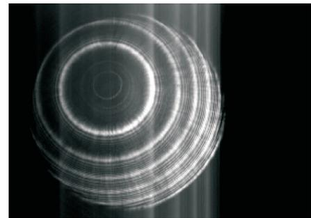
Fig. 2: A very preliminary Fabry-Perot fringe pattern using the E2V 30-11 ccd cooled at  $-130^{\circ}\text{C}$ .
