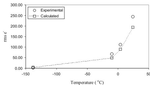
Fig. 3: The total noise of the E2V ccd as a function of temperature, (a) experimental and (b) calculated
