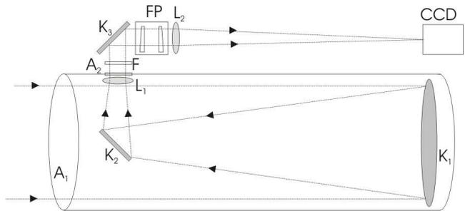
Fig. 1: Ray tracing in the Newtonian telescope with one of the two Fabry-Perot channels visible in this Figure. A1, A2: telescope apertures, K1, K2, K3: Mirrors, primary, secondary and another diagonal, L1, L2: Lenses, F: interference filter, FP: Fabry-Perot Interferometer
