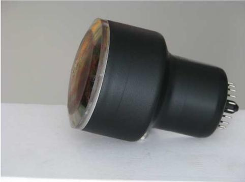
Fig. 2. The tested Photonis XP53B20 PMT.
