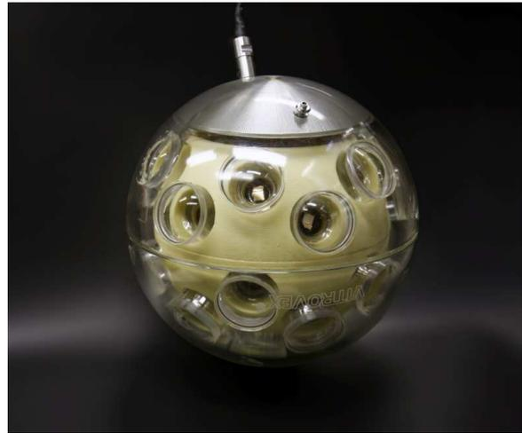
Fig. 1. Prototype of the MultiPMT optical module
