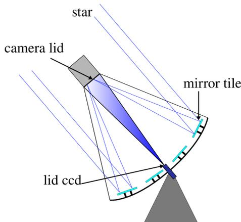
Fig. 1. Basic components and layout of the mirror alignment system (figure and procedure are based on [1]). Starlight is reflected by the individual mirror tiles of the reflector onto the PMT camera lid. A CCD camera takes pictures of these reflections, so called 'mirror spots'.
