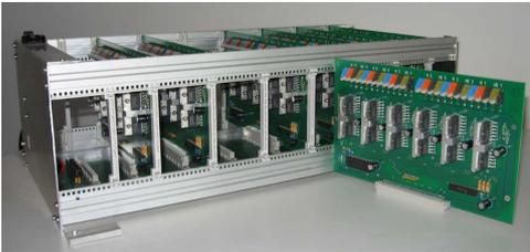
Fig. 3. Main electronics for one panel. A bus system connects the seven motor controller boards in the box. One of these boards is shown in the front.
