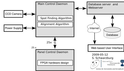
Fig. 4. Software components of the Mirror Alignment Control System
