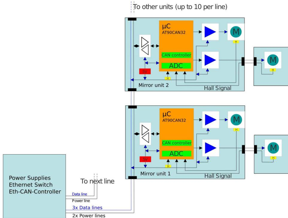
Fig. 6. Possible design of the CTA active mirror control system. Only parts on the telescope are shown. Starting from a central position in the dish, Ethernet to CAN converters are connected to several CAN busses, the actual number depends on the telescope design. Ten mirror units are connected to each CAN bus, each containing an Atmel microcontroller as the central control component.
