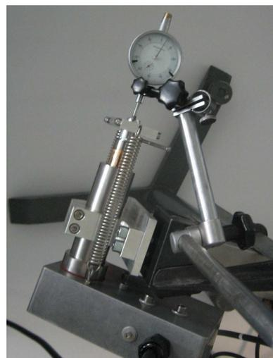
Fig. 5. Test setup to measure the accuracy during the long term tests.
