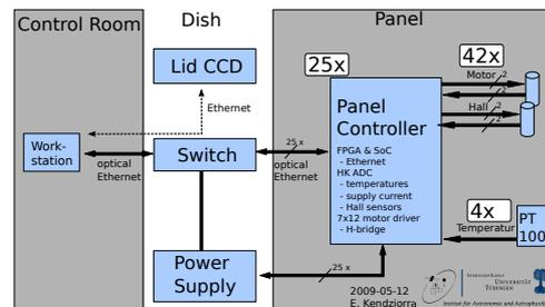
Fig. 2. H.E.S.S. 2 Mirror Alignment Block Diagram
