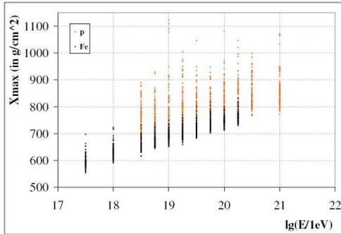
Fig. 1: The values of parameter  $X_{max}$  for the EAS depending on the logarithm of the primary particle energy, i.e. the particle initiating the EAS.
