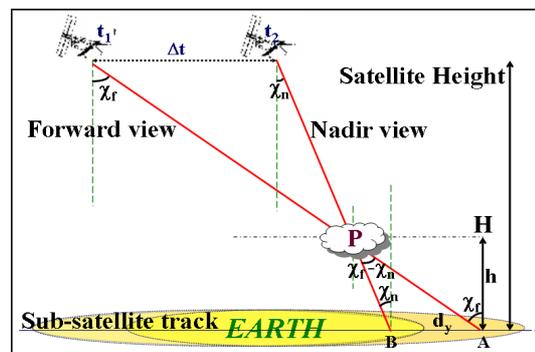
Fig.1. Two views of the same scene (stereo vision) obtained by moving the camera respect to the observed scene.
