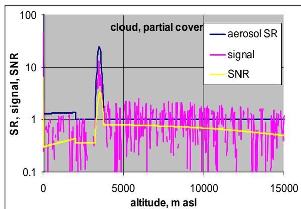
Fig. 5. Backscatter Signal and Signal-to-noise ratio for the proposed lidar, with one laser shot. See the text for explanation of the aerosol Scattering Ratio. Cloud coverage of the single pixel is 50%
