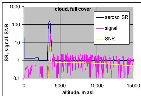
Fig. 4. Backscatter Signal and Signal-to-noise ratio for the proposed lidar, with one laser shot. See the text for explanation of the aerosol Scattering Ratio. Cloud coverage of the single pixel is 100%.
