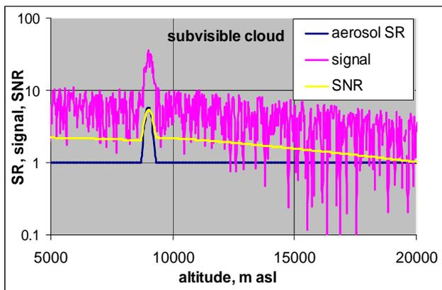
Fig. 6. Backscatter Signal and Signal-to-noise ratio for detection of the signal from high-altitude subvisible clouds and atmospheric molecular backscatter above and below the cloud. See the text for explanations for the aerosol Scattering Ratio.
