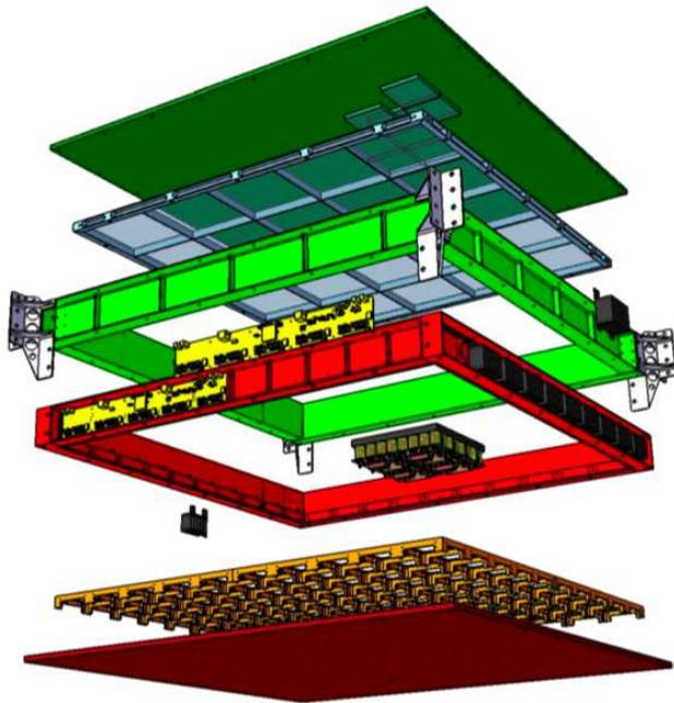
Fig. 1. Exploded CAD view of the CherCam mechanical structure
