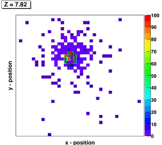
Fig. 2. High-charge particle event in the CherCam. Each pixel represents one PMT, where the color code indicates the number of Cherenkov photons seen. The Cherenkov ring and impact point of the incoming particle are clearly visible. The photons in the "halo" around the impact point correspond to the Rayleigh scattered photons. The reconstructed Cherenkov ring is represented by the ellipses.
