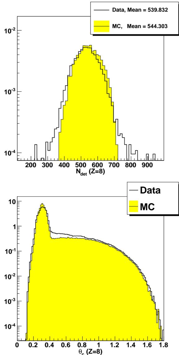
Fig. 3. Normalised distributions of the detected photon number (top panel) and the reconstructed Cherenkov angle (bottom panel) of these photons, for incident oxygen nuclei ( $Z = 8$ ). The filled areas correspond to simulated events and the thick lines to events reconstructed by the CherCam.
