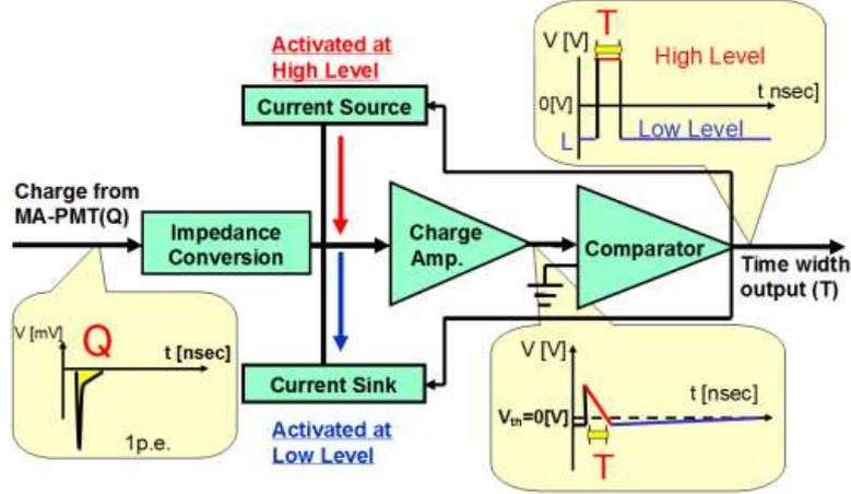
Fig. 3. Basic functional block diagram of the front-end ASIC (KI02).
