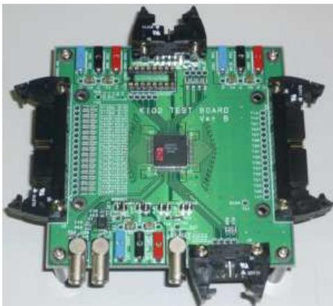
Fig. 5. Test board of the front-end ASIC KI02
