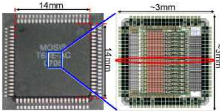
Fig. 4. 80pin QFP package (left) and a layout of KI02 ASIC (right).
