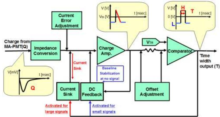
Fig. 8. Basic functional block diagram of the front-end ASIC (KI03).
