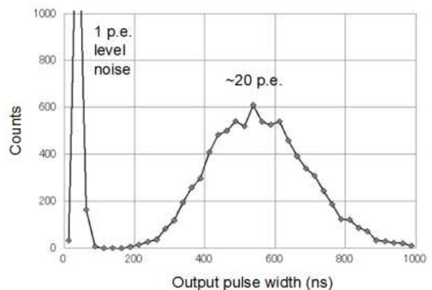
Fig. 7. Distribution of output pulse width in case PMT signals are fed into the KI02 ASIC.
