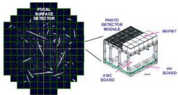
Fig. 1. Focal surface and Photo-Detector Module (PDM) of JEM-EUSO. Simulated air shower images with  $10^{20}$  eV are shown on the focal surface. The front-end ASIC will be mounted on the ASIC board which is connected to MAPMTs.
