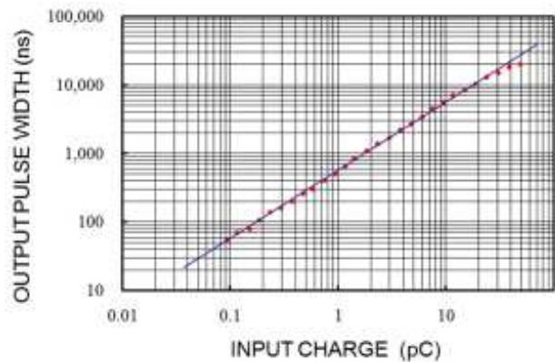
Fig. 6. Output pulse width vs. input charge.
