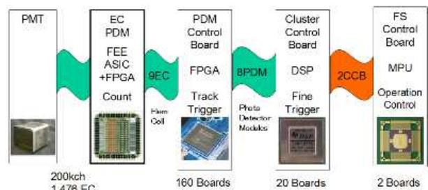
Fig. 2. Conceptual block diagram of JEM-EUSO data acquisition and trigger system.
