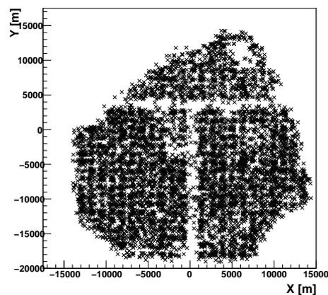
Fig. 1. The reconstructed core position distribution. The large blank region corresponds to the border of 3 part of SD array.[9] A few of unstable SDs also cause the small blank regions.
