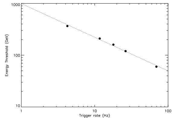
Fig. 5. Trigger rate vs energy threshold for photo-tube gains of 1, 2, 2.5, 3 and  $5 \times 10^6$ . Energy threshold decreases and trigger rate increases with increase in photo-tube gain.
