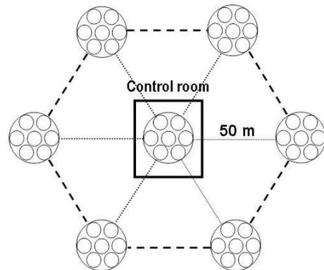
Fig. 1. Schematic layout of HAGAR array
