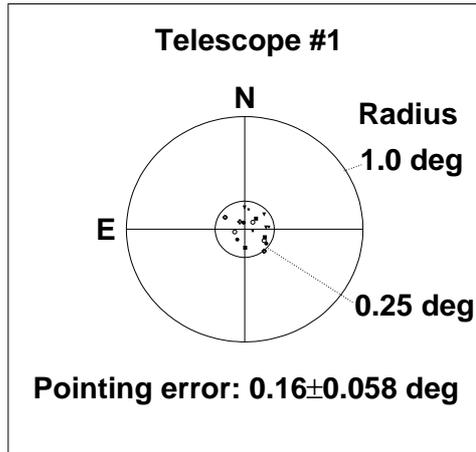
Fig. 3. Position of star images at the foci of 7 mirrors of the same telescope, Telescope # 1.
