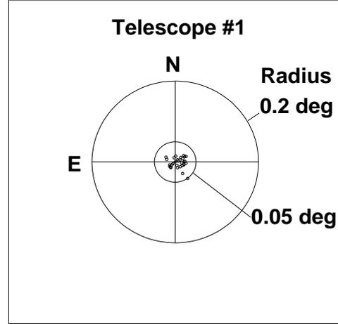
Fig. 2. A typical spread in the position of star images as seen in a guide telescope after applying pointing model. The stars are selected such that various elevation and azimuth angles are covered.
