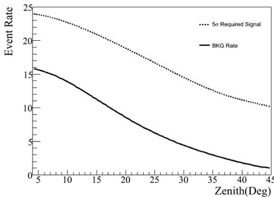
Fig. 5. The background event rate and the minimum signal event required  $5\sigma$  significance as a function of zenith angles for double front data.
