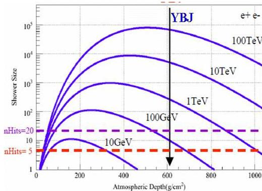
Fig. 3. The shower size as a function of Atmospheric Depth at different gamma ray initiated energy. If we set the trigger at 5Hit, the threshold can be greatly decreased in comparison with current trigger condition of 20 Hits.
