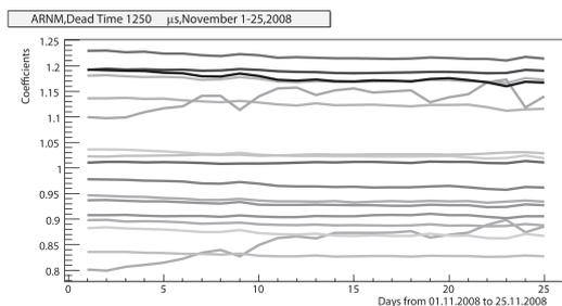
Fig. 6. Day-to-day changes of the channel coefficients of Aragats Neutron Monitor
