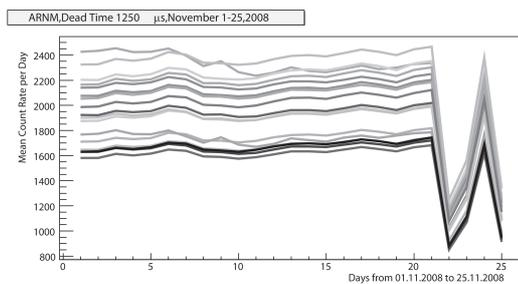
Fig. 5. Day-to-day changes of the mean values of Aragats Neutron Monitor; at November 22 there were power supply cut off
