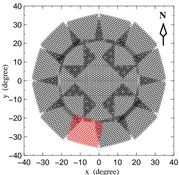
Fig. 6: WFCA FOV. Each circle represents the FOV of a PMT. The FOV is plotted in polar coordinate system, where (0,0) is the zenith.
