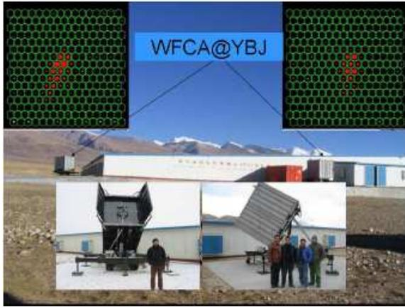
Fig. 7: Two WFCAs prototype telescopes operating at Yangbajing. The Cerenkov light images of one stereoscopic event observed by the two telescopes are shown at the top.
