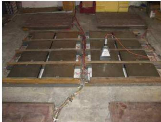
Fig. 5: SCDA prototype array (in the center of the figure) with 16 detector units operating at Yangbajing, a probe detector is deployed above for calibration purpose.
