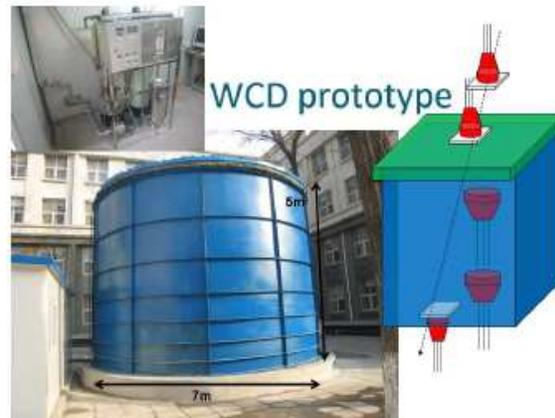
Fig. 4: A water Cerenkov detector prototype with the water circulation system shown in the top-left. The experimental configuration is shown in the right.
