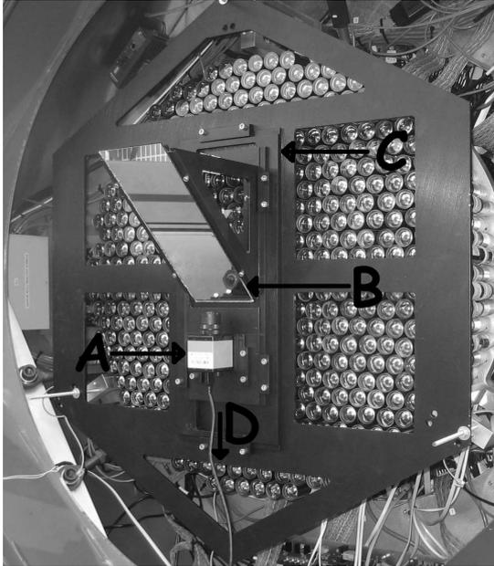
Fig. 2. A photograph of the alignment apparatus mounted on one of the VERITAS cameras. Arrow *A* indicates the CCD camera; *B*, the 45 degree mirror; *C*, the x-y positional stage and *D* the wire connecting to the data acquisition laptop (out of shot).
