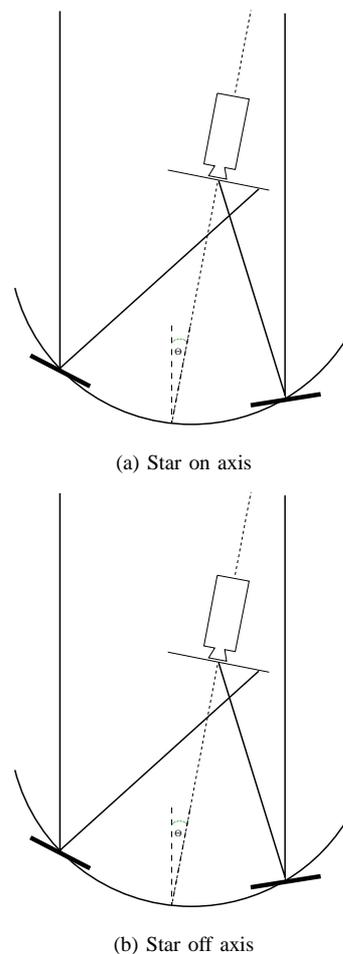
Fig. 1. An illustration of the raster scan method. In figure (a) the well-aligned facet will appear bright in the CCD image while the misaligned facet will be dark. In figure (b) misaligned facet will appear bright when the angle between the star and the telescope pointing direction is twice the misalignment angle of the facet.
