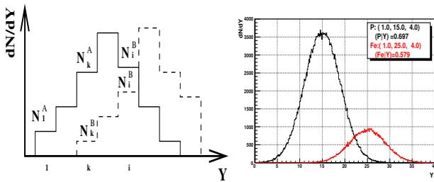
Fig. 3. Left: Definition of composition resolving parameters used in this work,  $(A|Y)$  and  $(B|Y)$ : Two histograms represent the distribution of variable  $Y$  (e.g. muon bundle energy loss in deep ice detector) for two types of primary particles (say proton and iron). Right: Particles A and B are represented by two Gaussian shaped distributions with the amplitude, mean and  $\sigma$  in the parentheses. Particle A and B each has 320000 and 80000 samples in this test.
