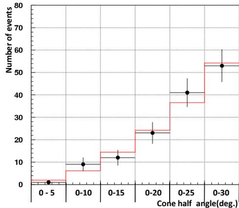
Fig. 1. Angular distribution of upmu-stopping events toward the Sun. Crosses indicate the data from SKI-III(2828.3 days) and the histogram indicates that of the atmospheric neutrino with normalization.
