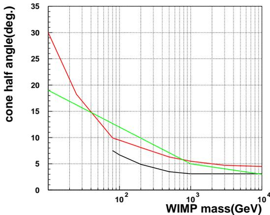
Fig. 4. Cone half angle which contain more than 90% of the signal from the WIMP annihilation is shown as a function of the WIMP mass [4]. Red line indicates the case 1), black one indicates the case 2) and green one indicates the case 3)
