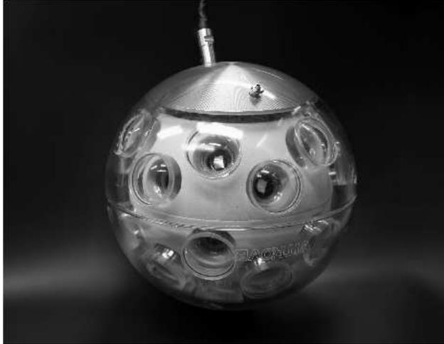
Fig. 1. Multi-PMT OM, developed in the KM3NeT design study project.
