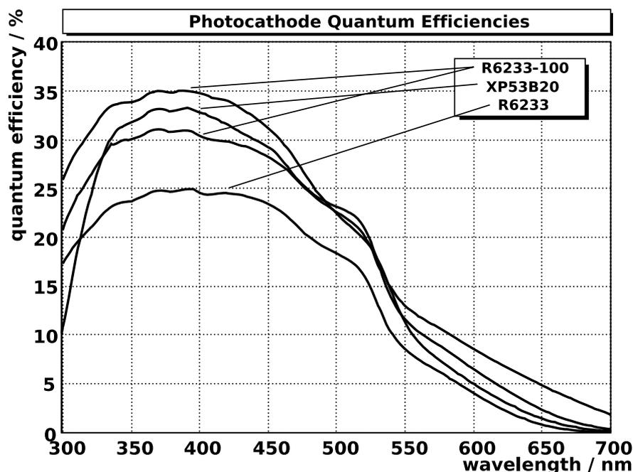
Fig. 4. Quantum efficiency for 3-inch PMTs. Maximum QEs vary between 31 and 35% for SuperBialkali / enhanced bialkali 3-inch PMTs. The lower curve denotes a standard bialkali-type R6233.
