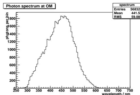
Fig. 1. Spectral distribution of Cherenkov photons after propagation through sea water (generated with Geant4, mean photon path length 30 m).
