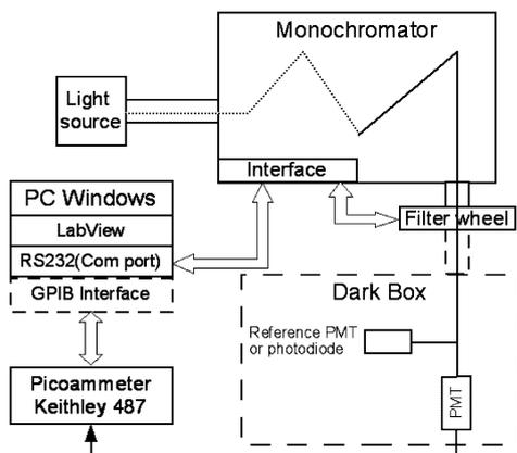
Fig. 3. Schematic of QE test setup
