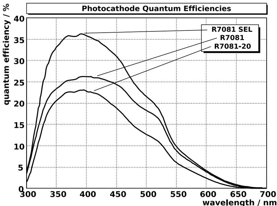
Fig. 2. Measured quantum efficiency for 10-inch PMTs. From top to bottom the results for R7081 SEL with a SuperBialkali photocathode and a maximum QE of 36%, the R7081 with a maximum of 26% and the R7081-20 with a maximum of 23% are shown.
