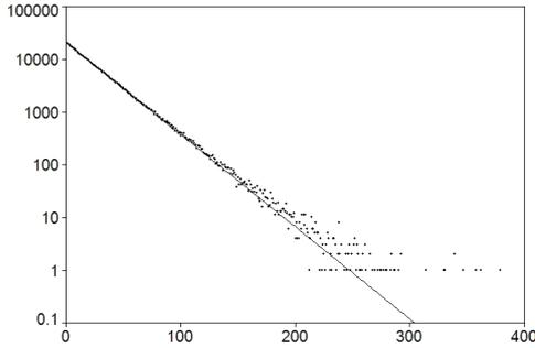
Fig. 4: The fitted exponential function on the real time differences between each two consecutive events, the obtained rate is 0.0403 Hz.
