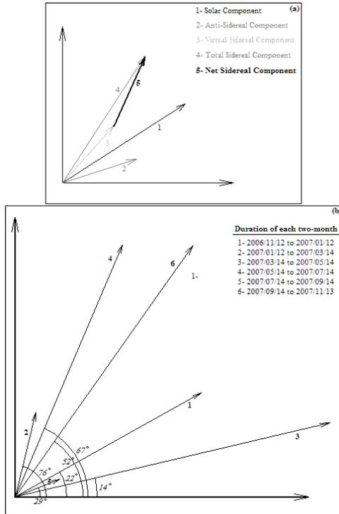
Fig. 2: **(a)**: Finding procedure of the net sidereal component. **(b)**: The obtained net sidereal components in six two-month durations.
