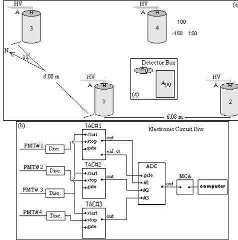
Fig. 1: **(Experimental setup)** Different parts of the figure respectively show **(a)**: schematic configuration of our detector array, **(b)**: data acquisition system and used electronic circuits, **(c)**(inside a): vertical ( $A_0$ ) and horizontal ( $A_{90}$ ) area surfaces of our detectors.
