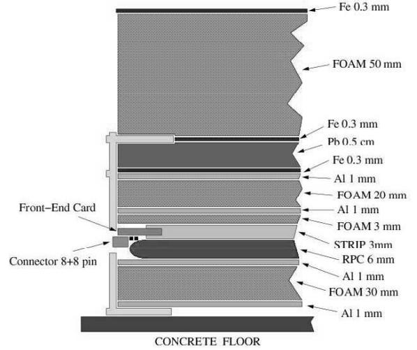
Fig. 2: Schematic cross-section of an ARGO-YBJ RPC
