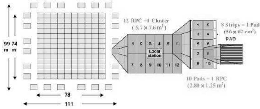
Fig. 1: Scheme of the ARGO-YBJ detector layout, with details of the detector geometry and structure.
