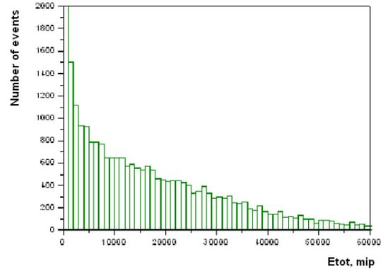
Fig. 2: Without any cut-off distribution of the total deposited energy in calorimeter initiated by a 1 TeV protons
