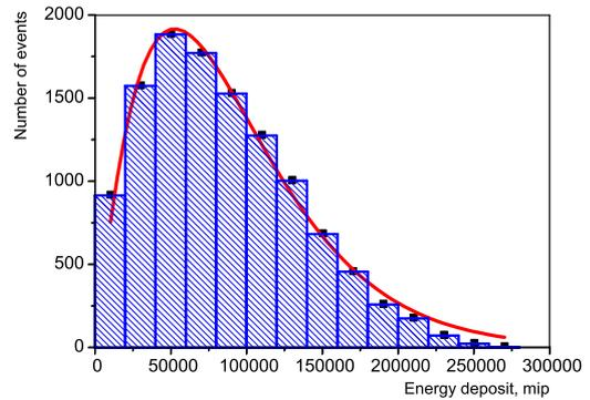
Fig. 3: Distribution of the total energy deposit for 2 TeV protons remaining after event selection (simulation result). The fitting function is KNO
