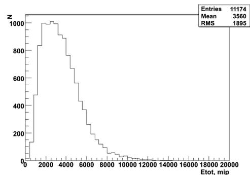
Fig. 4: Distribution of the total energy deposit for incident at  $0^\circ$  100 GeV protons remaining after event selection for the beam test data CERN 2003
