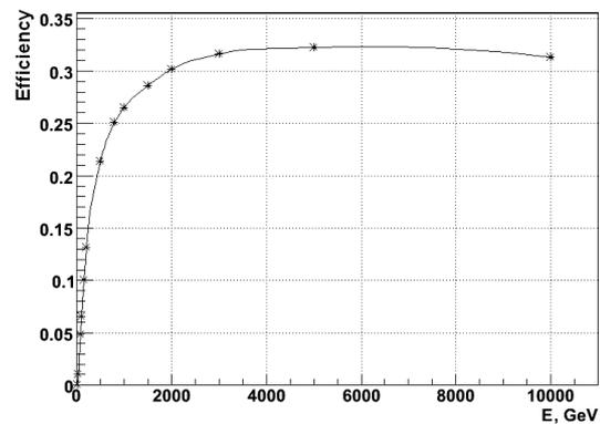
Fig. 7: Proton efficiency as function of primary energy
