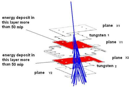
Fig. 1: The estimation method of starting point of the hadronic shower. For example in this fig shown the start of shower in first planes
