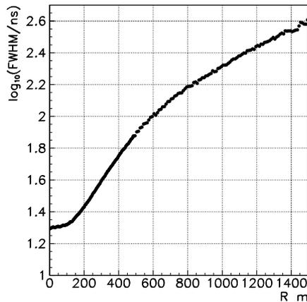
Fig. 3. Simulated width vs. distance function (WDF) for a single event.
