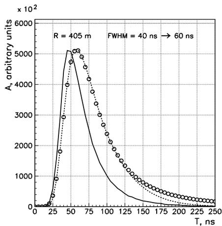
Fig. 1. Simulated apparatus distortion of the Cherenkov light pulse. Full curve - the CORSIKA simulated pulse, circles - the convolution of the simulated pulse and the apparatus function, dotted curve - fit of the distorted pulse by the expression (1).
