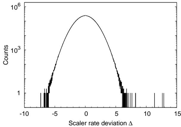
Fig. 2. Histogram of the deviations  $\Delta$  of the scaler counting rates. The distribution is Gaussian with a width of 1.4. Three candidate bursts are present above  $10\sigma$  which we looked at more closely to determine if they are due to GRBs.
