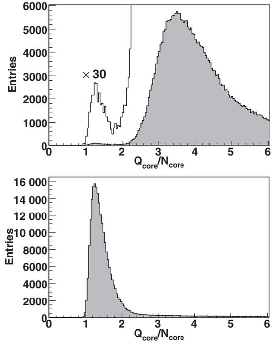
Fig. 3: Distribution of the energy density in the shower core weighted by the depth in the calorimeter ( $Q_{\text{core}}/N_{\text{core}}$ ) for negative (upper plot) and positive (lower plot) particles. In order to show better the left peak in the case of negative particles, the same distribution is also reported with the vertical scale multiplied by a factor 30 (white histogram).
