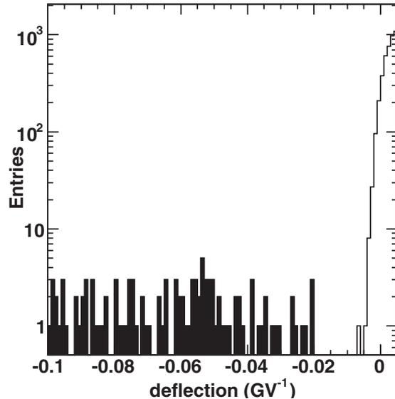
Fig. 2: Deflection distribution for down-going particles with a reconstructed MDR  $\geq 850$  GV which did not produce an electromagnetic shower in the calorimeter. The good separation between positive and negative particles can be seen, as well as the spillover of positively charged particles into the negative deflection region. The shaded part of the histogram corresponds to particles selected as antiprotons.
