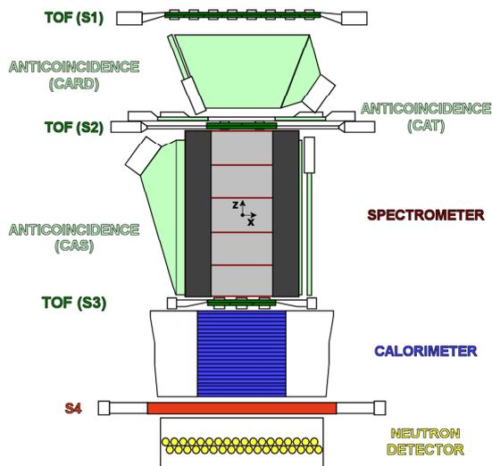
Fig. 1: Schematic drawing of the PAMELA detector showing the sensitive areas of the various sub-systems to scale, in a longitudinal section.
