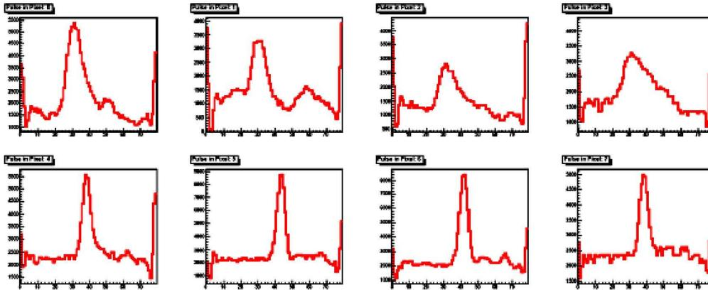
Fig. 4. An event seen by the 4 G-APDs (top) and in the surrounding 4 PMTs (bottom row), digitized by a 2 Ghz F-Adc. The G-APD signals are clipped by 50 Ohm coax cables to  $\approx 3$  nsec. Pickup peaks at start and end by multiplexer.
