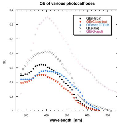
Fig. 2. QE ( $\lambda$ ) for different sensors
