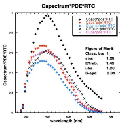
Fig. 3. PDE ( $\lambda$ ) folded with the Cherenkov spectrum and the optical parameters (R,T,C) of the Magic telescope
