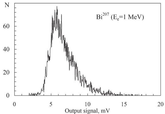
Fig. 4: Amplitude spectrum of structure-output signals produced by relativistic electrons ( $E_e = 1$  MeV) emitted by a  $\text{Bi}^{207}$  source. The distribution asymmetry shows the Landau law behaviour of losses.
