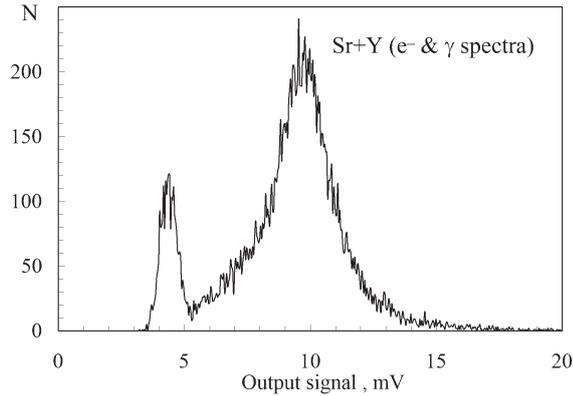
Fig. 5: Amplitude spectrum of output signals produced by electrons and  $\gamma$ -rays emitted by a strontium/yttrium (Sr+Y) source.
