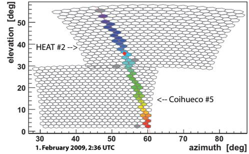
Fig. 3. This shower was recorded by HEAT telescope #2 and Coihueco telescope #5. The relative arrival time of the fluorescence light is coded in the colour of the pixel. The solid line is a fit of the shower detector plane.
