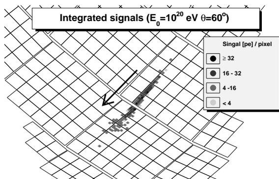
Fig. 4. Image on the focal surface detector for the same typical EAS as in Fig. 3. The time-integrated signal in each pixel is shown in digitized scale. The blocks correspond to the individual MAPMTs. The arrow indicates the direction of the movement of the signals.
