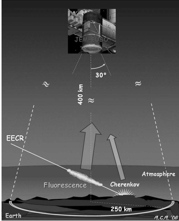
Fig. 1. Illustration of EECR observation principle in the JEM-EUSO mission. For the telescope at  $H_{\text{orbit}} \sim 400$  km altitude, the main signals are fluorescence photons along the EAS track and Cherenkov photons diffusely reflected from the Earth's surface.
